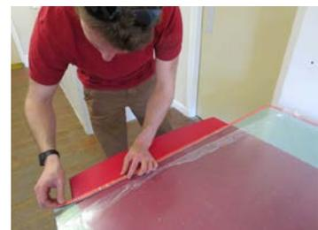
Step 5: Peel away the red backing on the magnetic tape.
