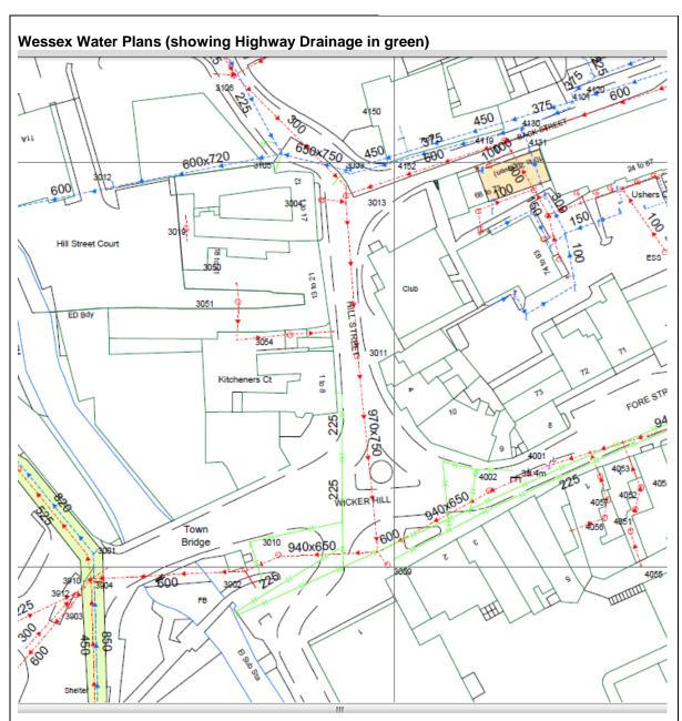
All highway drainage has been jetted and CCTV surveyed. Gullies on Hill St are connected via weir walls into the WW foul culvert and were proven with dye. All other highway drainage found to be in good condition. Wessex Water have cleaned/surveyed their systems and found them free of defects. With both systems there was a possibility of silt build up at points, but this is hard to confirm as it would have been cleared by jetting.
