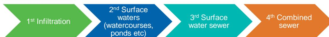
However, there are instances where infiltration to ground is inappropriate and soakaways will not work. The groundwater level is a major factor in determining whether a soakaway is viable or not. A high groundwater table is an indication of limited infiltration potential.
