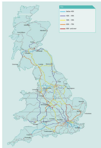
Figure 6.2 Actual freight train utilisation of WTT paths on key freight sections. Source: Network Rail
