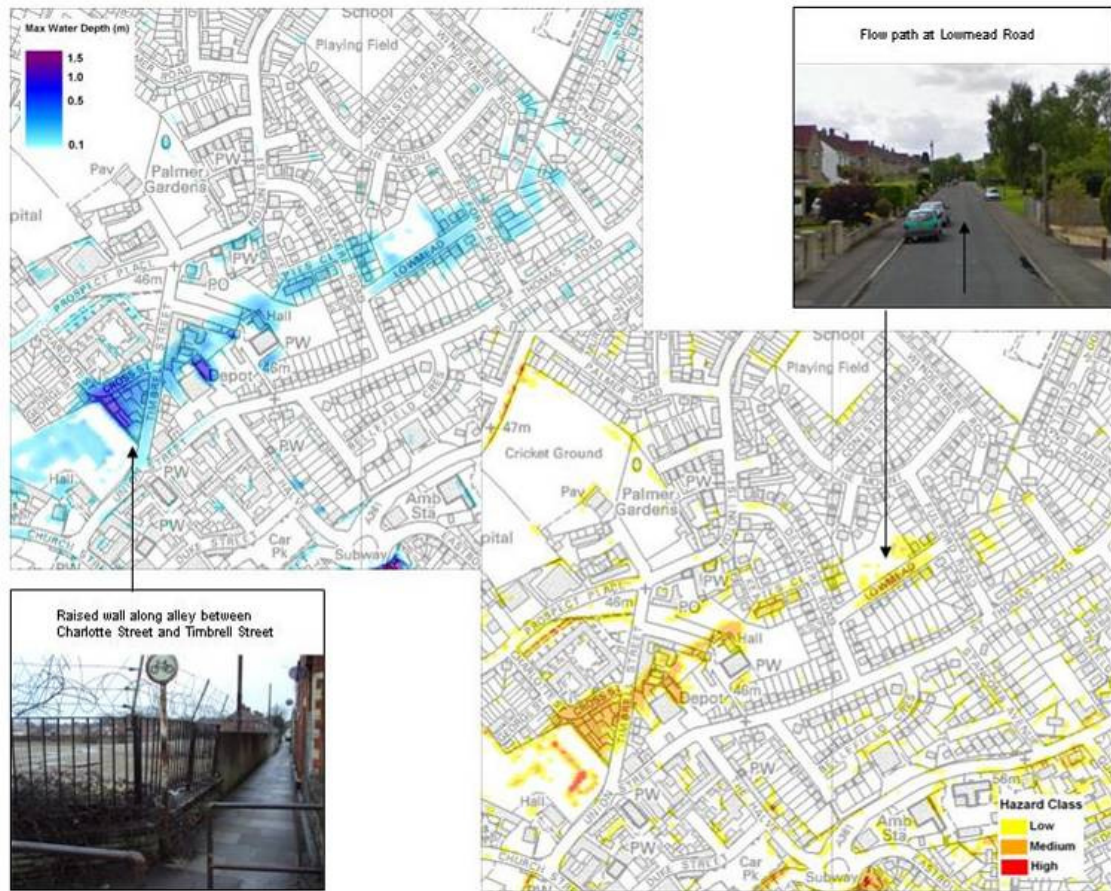
Figure 6-2: Pluvial modelling results (maximum potential depth and hazard) for the 1% AEP rainfall event including an allowance for climate change for the Timbrell Street Area
