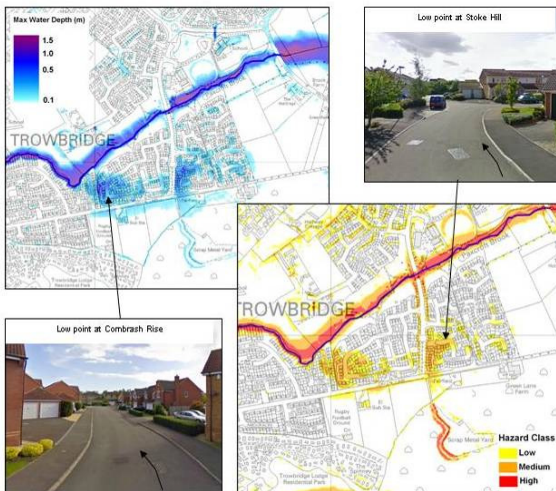
Figure 6-3: Pluvial modelling results (maximum potential depth and hazard) for the 1% AEP rainfall event including an allowance for climate change for the Green Lane Area.
