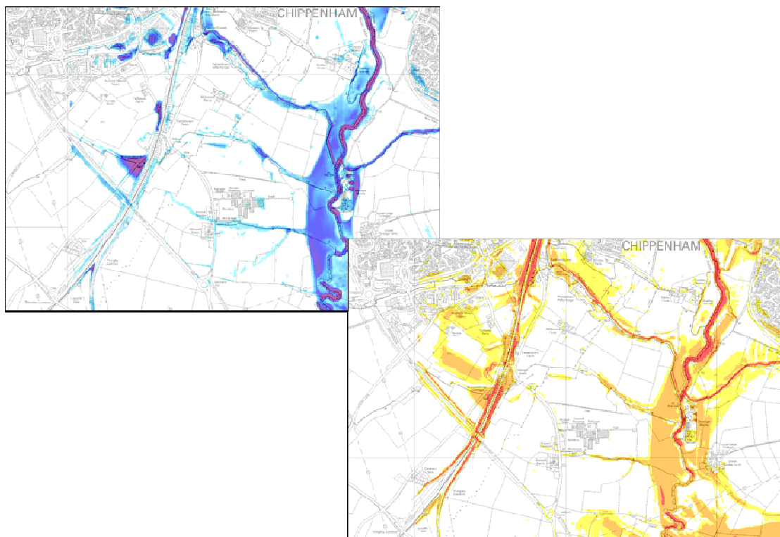
Figure 5-11: Pluvial modelling results during the 1% AEP rainfall event, inclusive of climate change (maximum depth and hazard) for the Patterdown Area
